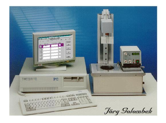
Device and method for measuring the curing and the condensation properties of reaction resins (e.g. aminoplast, epoxy, polyester, polyurethane etc.) of impregnated papers, fleeces, tissues etc.
