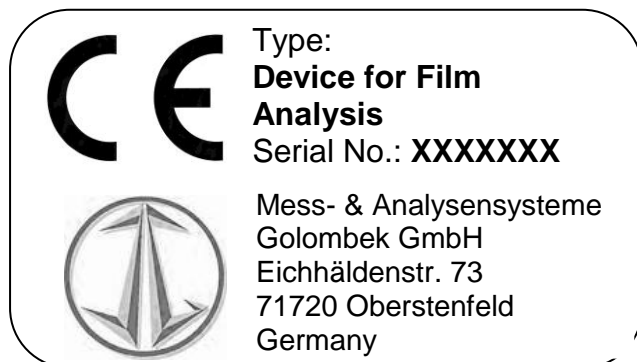
Figure 1: __Type plate with CE marking
